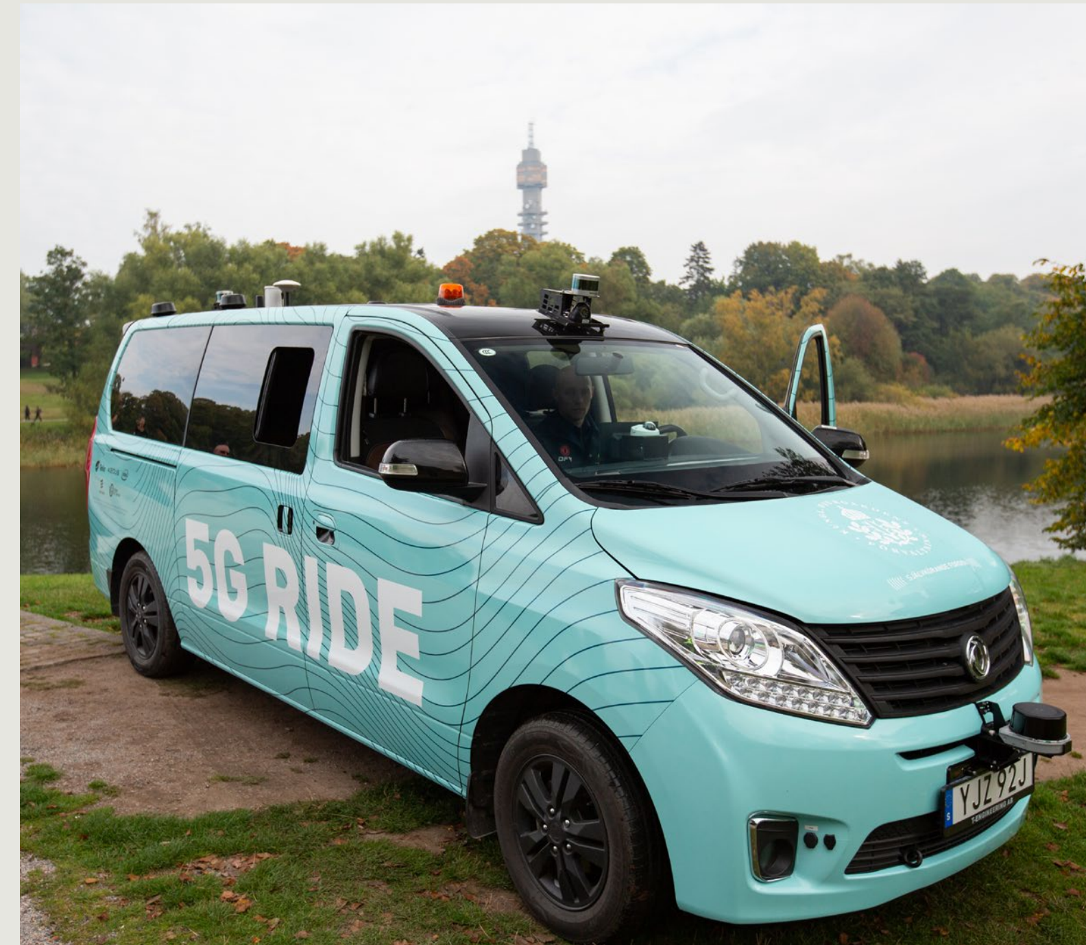
The 5G Ride project focuses on how 5G and control towers can enable the safe introduction of self-driving, electric buses in urban areas. This pilot was run in Djurgården in Stockholm, Sweden.
