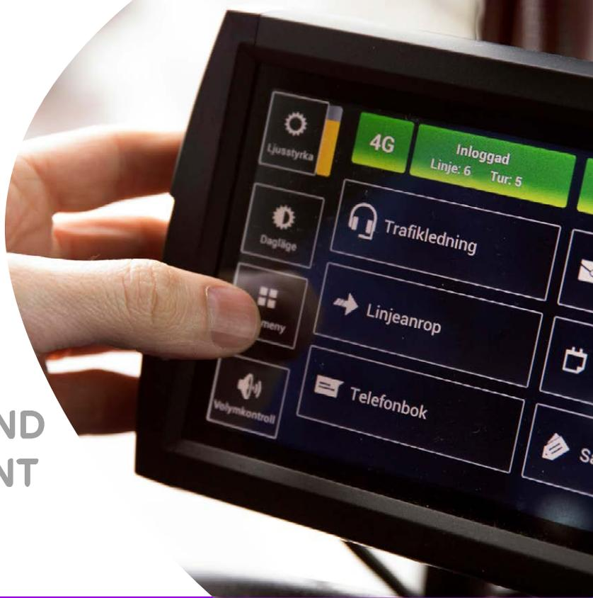
Improve communication between drivers and traffic management by adding VoIP voice communication to your vehicle. A screen, microphone and speaker are placed by the driver's seat, and the conversation can begin.
